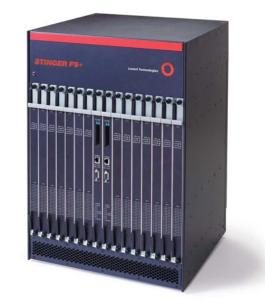
The Stinger FS+ utilizes multiple high performance, minimum delay, redundant ATM and IP switching fabrics for supporting the highest speed network application requirements of today.
